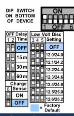
**DS1-DS2** sets delay between Off Trigger and Relay OFF. OFF is for install testing or pure relay functionality without time delay
