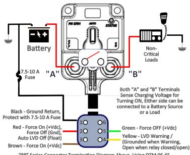
"88" Series Connector Termination Diagram Above, Using DTM 06-6S. Customer Supplies DTM04-6P. For "87" Series Products, Tinned Copper Wires Provided (Per Colors)
