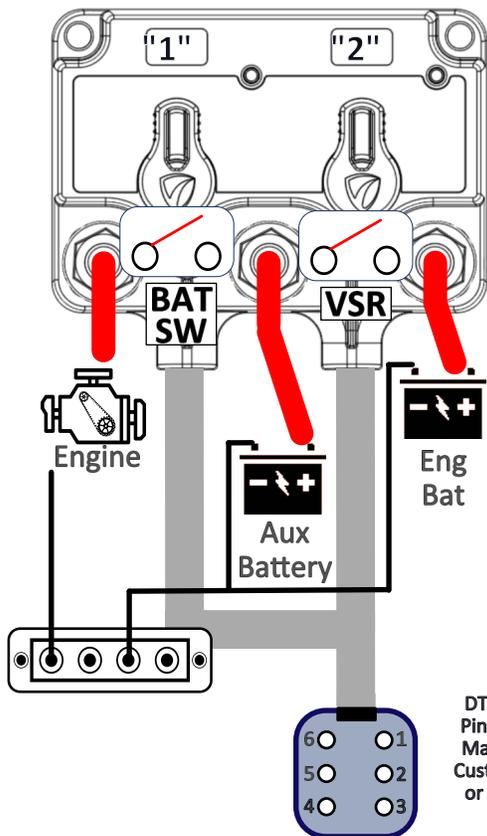
Depicted with manual override knobs in all locations. Availability of manual override knob for either relay position determined by the part number. See part number guide for further details.
