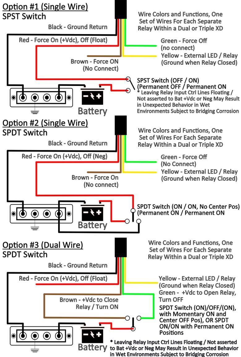
**Fig 2 - Mechanical Only Contactor Option**
