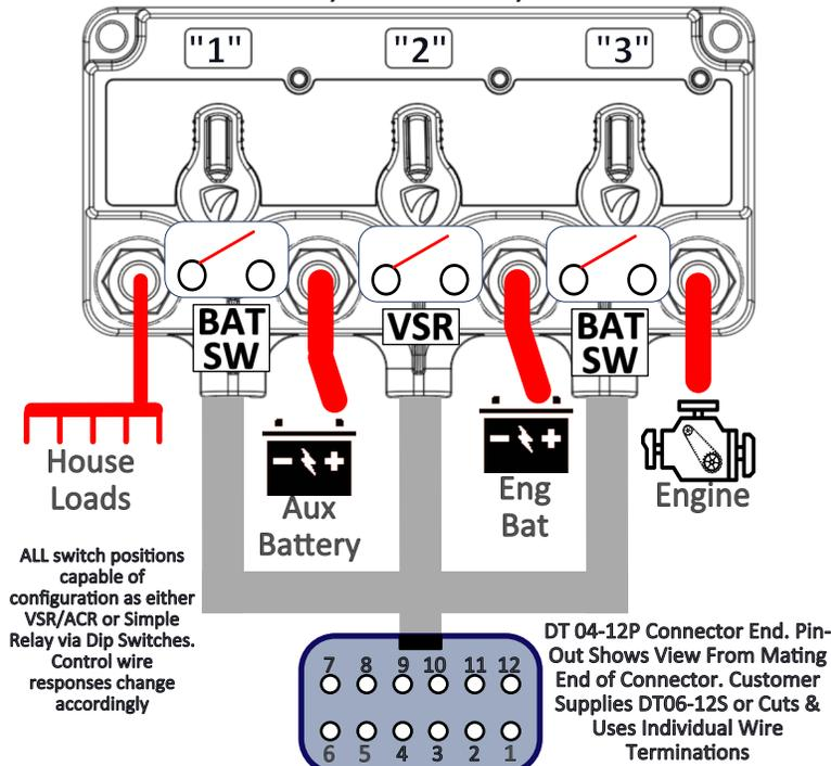
**6 Pin DT Connector Functions (Fig 10)**
