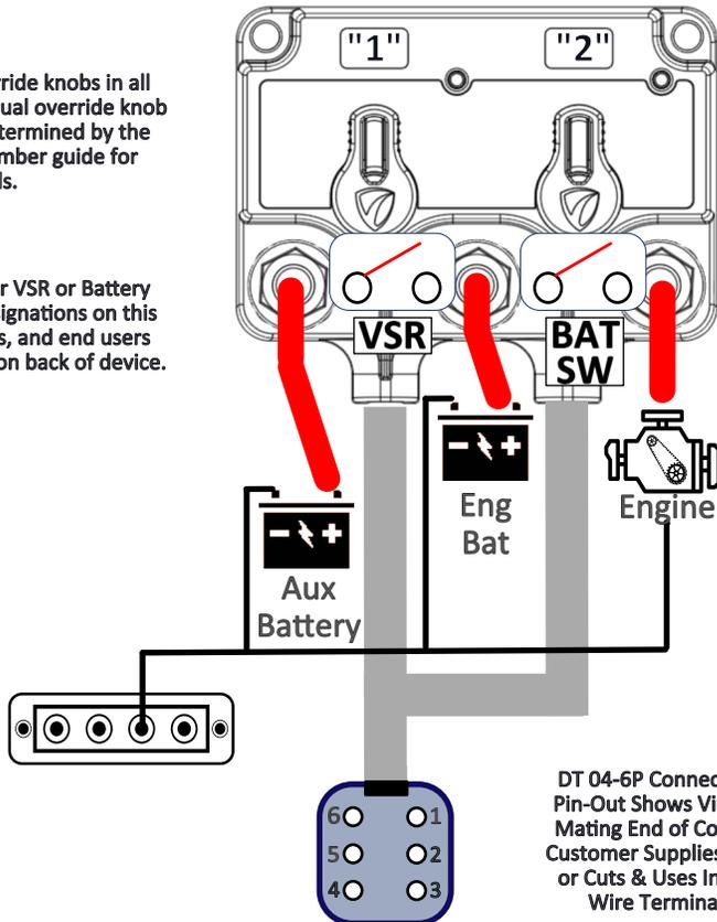
DT 04-6P Connector End. Pin-Out Shows View From Mating End of Connector. Customer Supplies DT06-6S or Cuts & Uses Individual Wire Terminations
