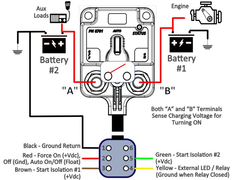
A) 88xx-xxxx Part Numbers Use a DTM 06-6S Connector End. Customer Supplies DTM04-6P or Cuts & Uses Individual Wire Terminations.
