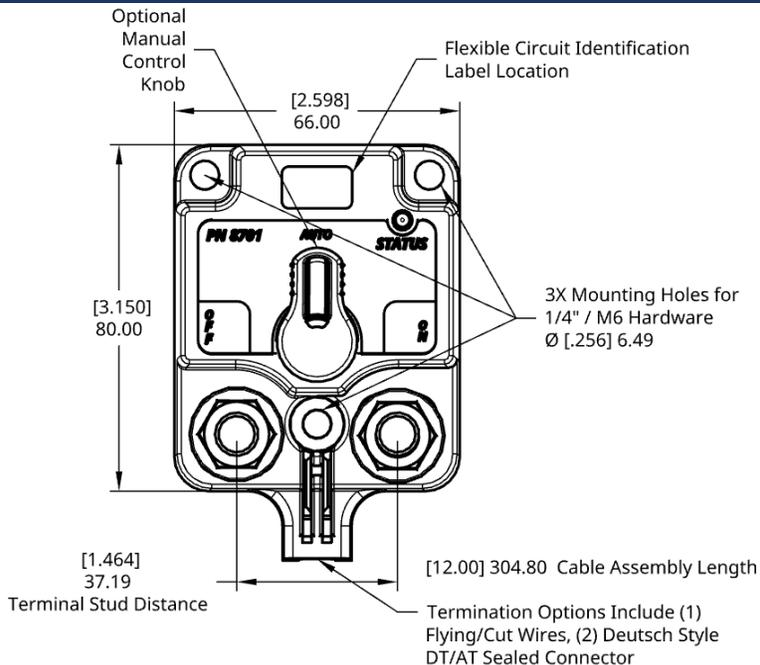
2X M10 x 1.5 Stainless Steel High Power I/O Terminals & Serrated Flange Nuts.
