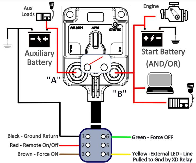
DTM 06-6S Connector End, Customer Supplies
