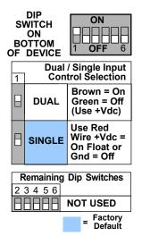
**DS1** sets single or dual input control. Dual mode is for separate +Vdc inputs for OFF (green wire) and ON (brown wire) Single mode is for +Vdc ON (red wire) and floating / Gnd (red wire) for OFF
