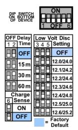
**DS1-DS2** sets delay between Off Trigger and Relay OFF. OFF is for install testing or pure relay functionality without time delay
