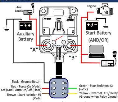
DTM 06-6S Connector End. Customer Supplies DTM04-6P or Cuts & Uses Individual Wire Terminations
