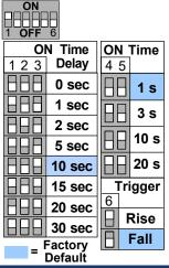
DS1-DS3: Determines time delay between registering a Trigger signal on the yellow control input and the Output of device turning on (+Vdc) per table to the left. Each combination of three dip switches (on or off) result in a unique On time Delay DS4-DS5: Determines the Output ON duration before the device automatically turns the output OFF per table to the left. Once output is OFF, it can not be turned on until a new Trigger signal is received.
