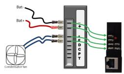
*3b. Move existing blade connectors to connection block*
