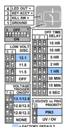
**DS1-DS3** sets delay between Off Trigger and Relay OFF. 0 SEC is for install testing or pure relay functionality without time delay
